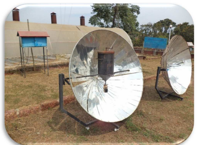
CNSL Extraction using solar concentrating cooker
